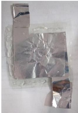
Fig. 6. FSR based on the prototype
