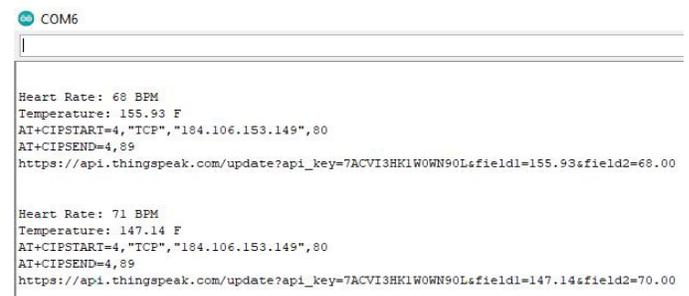
Fig. 12. Hardware results on Arduino Serial Monitor
